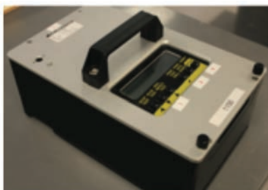
An example of the BOT-3000 Tribometer, one of the primary test methods used for measuring ANSI/NFSI B101.3. Source: Tile Council of North America.
