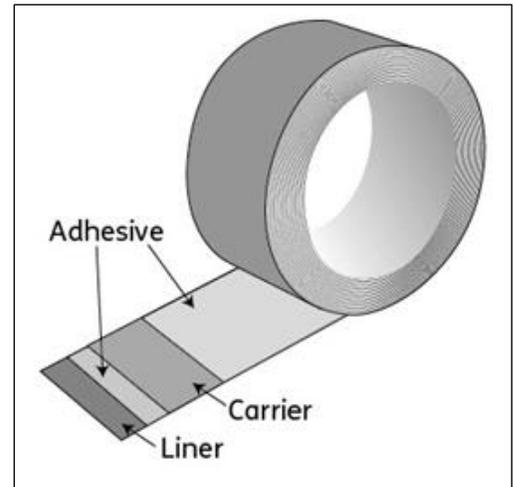
The following properties are typical for a Double Coated Film:
