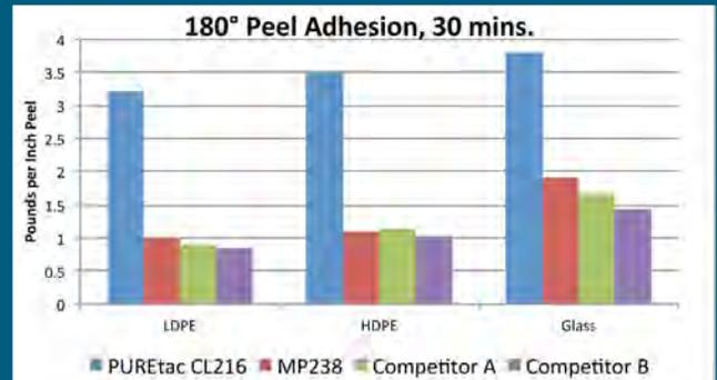
The chart above shows how Mactac PUREtac CL216 outperforms the competition for secure adhesion after the 30 minute peel test, showcasing the adhesives' superior long-term aggressiveness.
