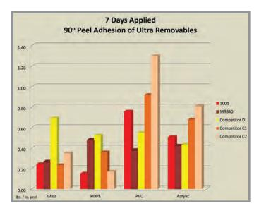
The chart above compares Mactac's two ultraremovable adhesives, 1001 and MR840, to three competitor products. With removable adhesive, the lower the peel value, the simpler it is to remove the label. With this in mind, it's easy to see that Mactac ultra-removable adhesives consistently outmatch the competition.
