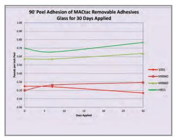
The chart above compares 90 degree peel-adhesion of new and current Mactac removable adhesives' performance over the course of 30 days. MR840 and MR860 deliver consistent peel whether removal happens immediately or after a month of adhesion.
