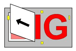
Remove the AT at a steady speed, at a cleaving angle of between 0 and 30°.
