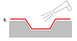
Once 100% of the vinyl is in contact with the surface, **heat the vinyl with heat gun or hot air blower** (air temperature: 350-400°C). This reinforces the initial adhesion. The decoration should not be exposed to temperatures lower than 10° C during the first 3-4hours.
