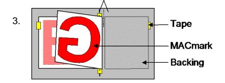
For surfaces of this kind, it is absolutely necessary to apply AT to the lettering or logo. Position the lettering or the logo WITHOUT REMOVING THE BACKING by using a piece of positioning tape at each end.
