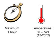
Mactac recommends weeding as soon as the shapes have been cut out. This is because the thickness of the adhesive layer could result in it "resealing" itself if the vinyl is left for several hours before weeding, or if it has been exposed to temperatures above 78° F(25°C).
