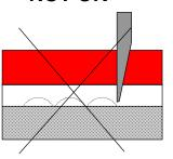
Applying too much pressure when using a blunt knife could result in the knife bouncing off the backing paper, which means that the adhesive will not be cut all the way through.
