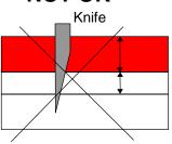
If cuts are too deep, then the backing could split when the letters or logos are being transferred onto the MACtransfer tape.
