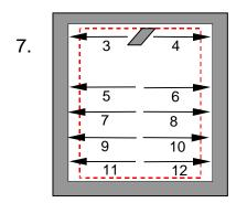
Squeegee the last 3 inches of the top edge working from the center outwards, to the left and then the right. Continue to squeegee horizontally moving from the center outwards with overlapping movements. Check that no pockets of water have been trapped. If this is the case, scrape from the center to the edge in order to squeeze it out. Wipe the vinyl and the edges.
