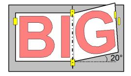
Fold the hinge back making sure that you leave a space between the MACmark vinyl and the substrate surface (angle of ±20°) in order to avoid it sticking too soon.
