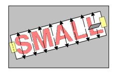
Position the lettering or the logo once again on the spot marked by the piece of positioning tape. Squeegee quickly and firmly from the center outwards in overlapping movements.
