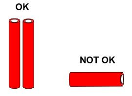
Any partly used rolls should be kept upright or hung on racks. At no time should they be placed on their sides as this could lead to a large matt section appearing throughout the entire roll.
