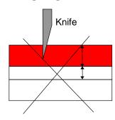
If the cut is not deep enough (the vinyl and/or if the adhesive is not cut all the way through), the letters and logos that you have cut out could be pulled away during stripping.
