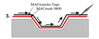
Apply MACmark 9800Pro using MACtransfer application tape through the 3 dimensional surface. Use your finger or a stiff bristle nylon brush, (cut off to approximately <sup>3</sup>/<sub>4</sub>") along the lines of the corrugations to make the vinyl conform to the curved surface.
