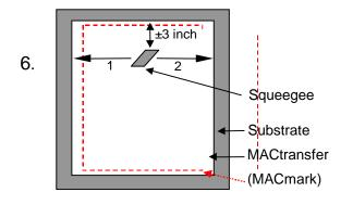
Squeegee horizontally, working from the center outwards to the left and then the right stopping  $\pm 3$  inches from the top edge of the vinyl. Apply enough pressure to squeeze out any water trapped between the MACmark adhesive and the substrate surface.
