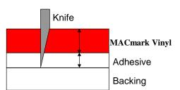
Cut to the correct depth. The knife should cut all the way through the vinyl and the adhesive.
