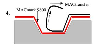
Remove the AT. Prick and squeeze out any air bubbles that appear.
